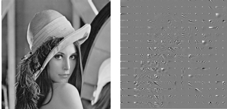
Figure 1: An image and its DCT applied to frames of 16 \times 16 pixels. A grey level was added to the DCT, since its coefficients can be negative.
