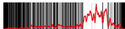
(c) The intensity profile shows the diffuse reflection as well as the specular reflection at the right
